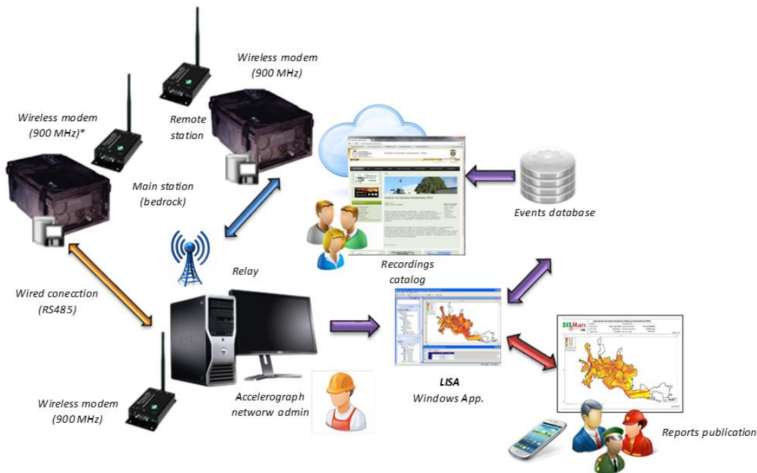
Figure 1. Structure and main components of LISA.
