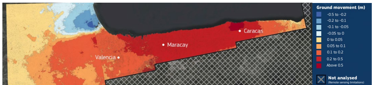
Figure 5. Permanent ground displacement associated with the June 24, 2026, Venezuela earthquakes, measured on June 25, 2026. Source: EU Copernicus.
